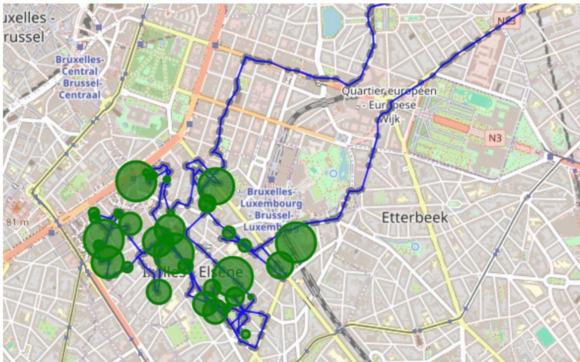
Figure 3 Map showing the matched GPS trace for a day of deliveries, and the matched stops. The size of the green circles shows the relative time spent at the stop. This route is in the neighbourhood called "Matonge", a particularly difficult area for deliveries, due to high parking constraints and high levels of congestion.
